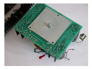
Now the Psu caps can be replaced. The revision of the amplifier boards is not different from the MKI, in some cases the MK II has already the input and feedback modification implemented. Rebuilt in reverse order.
