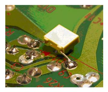
If you want an input-sensitivity of 0 dBm (0.775 mV), 1mWatt in 600 ohms, which is standard, replace R11 with 12 Ohm. If you leave R11 in place the input-sensitivity will be 0.5 Volt.
