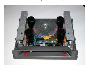
The unit will looks like this. Remove the amplifier boards with a long Philips (posidriv) screwdriver; be careful not to make contact with the components on the boards. Remove (loosen) the connectors on the boards with small pliers. Make notes, or pictures.
