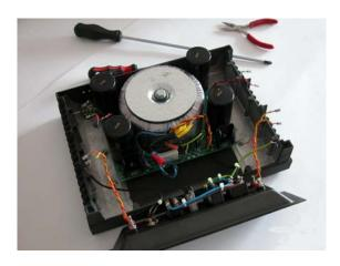
Remove the connectors from the PSU, make notes, or pictures! There is no need for soldering here. There are four large posidriv screws around the transformer, remove those. Be careful, sometimes they are a little bit covered by the transfo, lift the Psu Pcb to loosen those screws.
