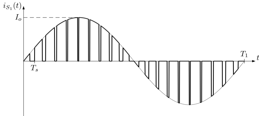
Figure 3.6: Current through MOSFET S_1 with a sinusoidal current source as load.
