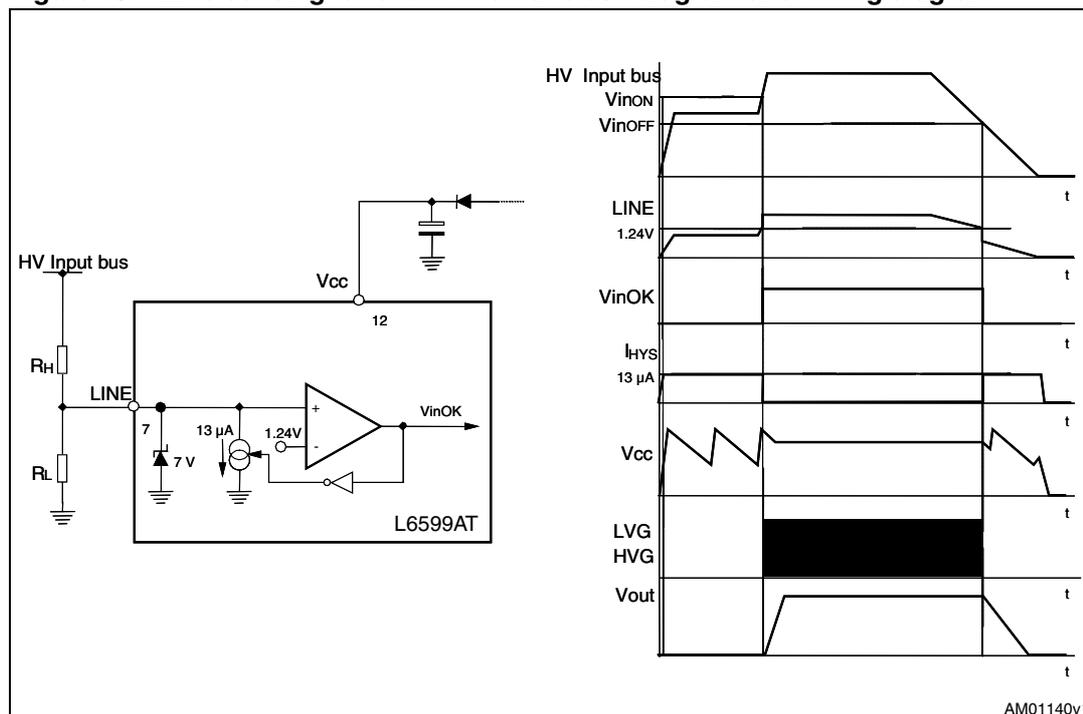
With reference to [Figure 11](#), the following relationships can be established for the ON ( $V_{inON}$ ) and OFF ( $V_{inOFF}$ ) thresholds of the input voltage:
