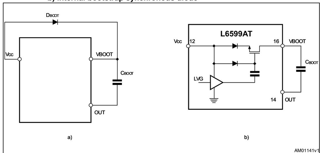
The diode prevents any current flowing from the VBOOT pin back to  $V_{CC}$  if the supply is quickly turned off when the internal capacitor of the pump is not fully discharged. To drive the synchronous DMOS a voltage higher than the supply voltage  $V_{CC}$  is necessary. This voltage is obtained by means of an internal charge pump ([Figure 14b](#)).
