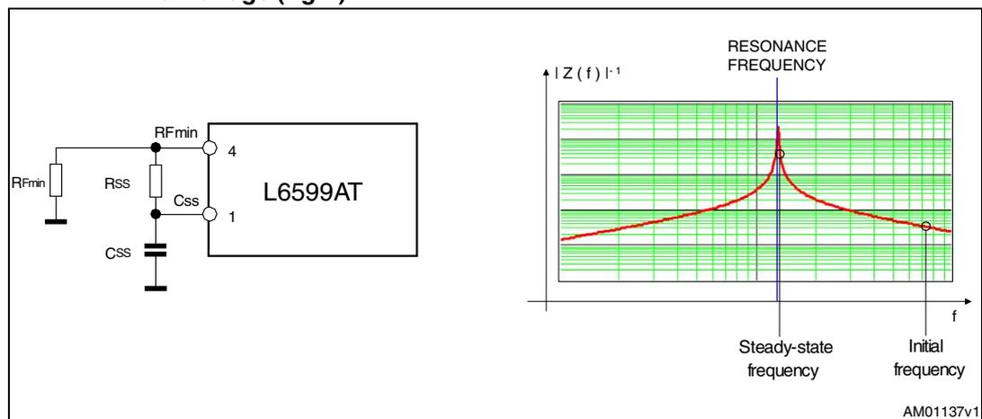
As a result, the average input current increases smoothly, without the peaking that occurs with linear frequency sweep, and the output voltage reaches the regulated value with almost no overshoot.
