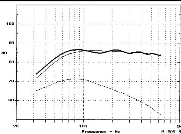
**FIGURE 18:** High-Q woofer on 43Hz tapered pipe: cone output, pipe output, and system response (bold).
