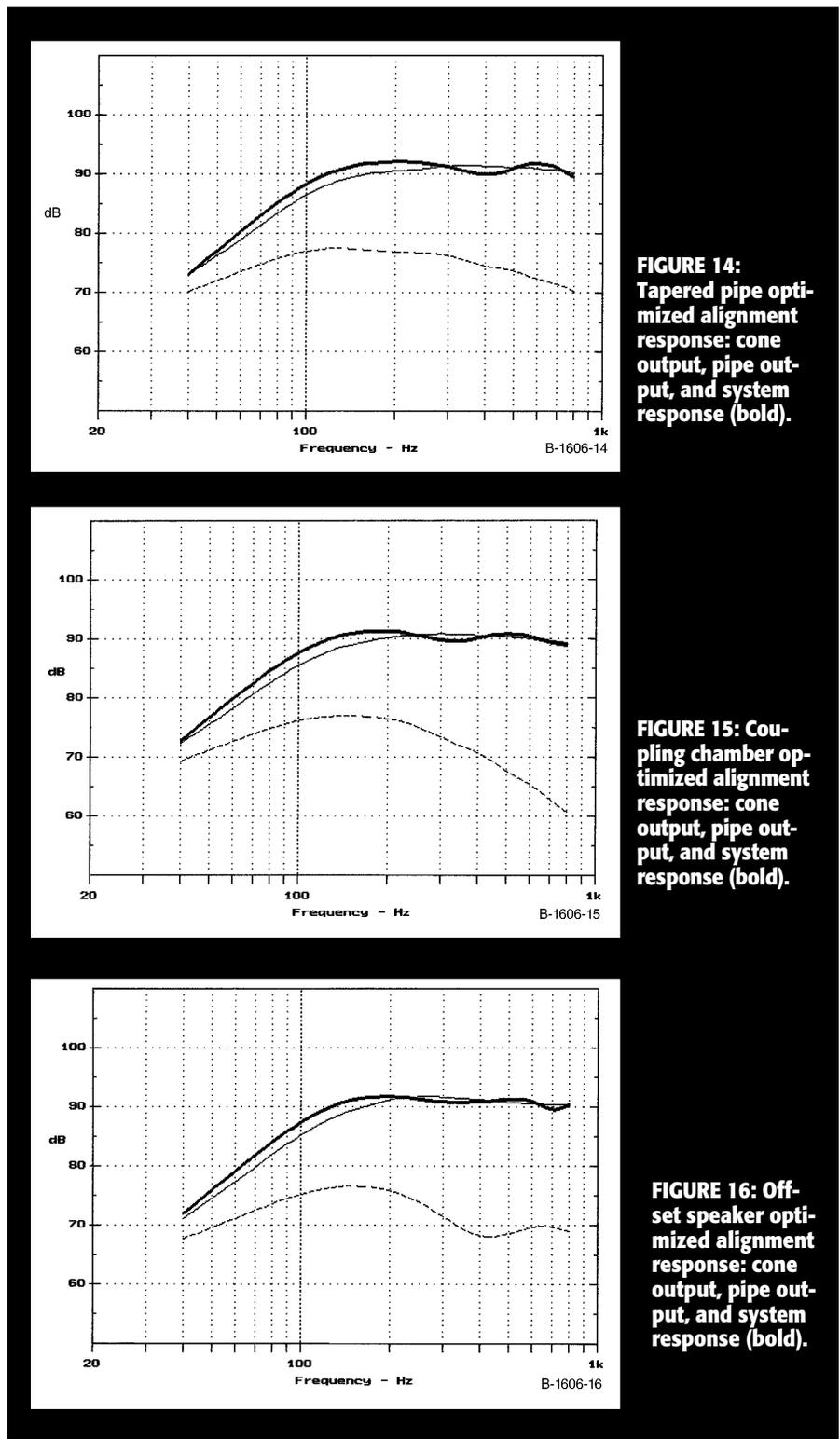
**FIGURE 14:** Tapered pipe optimized alignment response: cone output, pipe output, and system response (bold).
