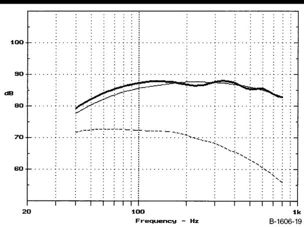
**FIGURE 19: Vifa P17WJ on 74Hz tapered pipe: cone output, pipe output, and system response (bold).**
