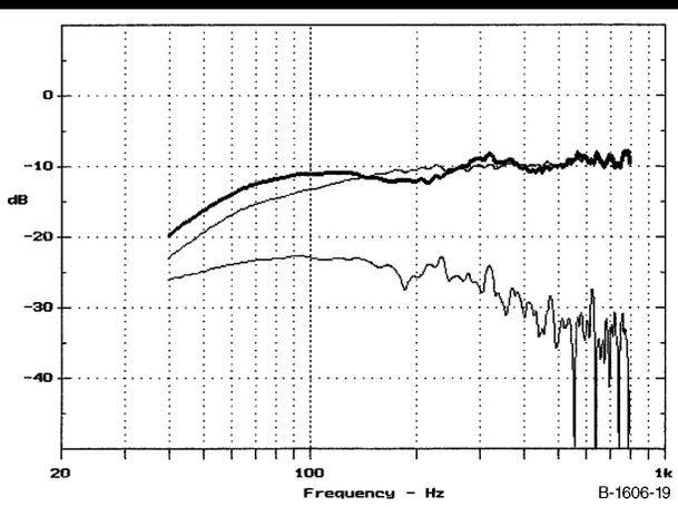
**FIGURE 20: Vifa P17WJ on tapered test pipe: cone output, pipe output, and system response (bold).**
