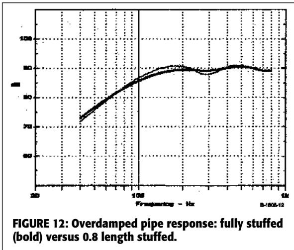
**FIGURE 12: Overdamped pipe response: fully stuffed (bold) versus 0.8 length stuffed.**
