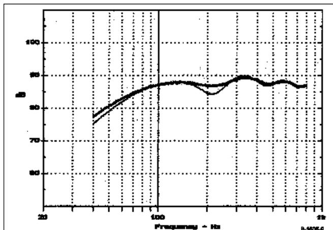
**FIGURE 9: System response: flared versus tapered (bold).**
