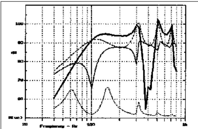
**FIGURE 3:** Response of loudspeaker on undamped straight pipe. Impedance (bottom), cone output, pipe output, and system response (bold).
