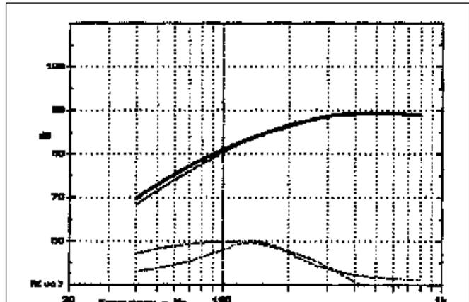
**FIGURE 4C:** Response of loudspeaker on straight pipe with heavy damping. Impedance, cone output, pipe output, and system response (bold).
