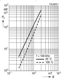
Relative core losses versus temperature (measured on R34 toroids)
