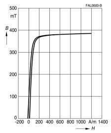
DC magnetic bias of P, RM, PM and E cores  $(\hat{B} \le 0.25 \text{ mT}, f = 10 \text{ kHz}, T = 100 ^{\circ}\text{C})$
