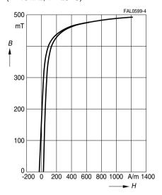
DC magnetic bias of P, RM, PM and E cores  $(\hat{B} \le 0.25 \text{ mT}, f = 10 \text{ kHz}, T = 25 ^{\circ}\text{C})$
