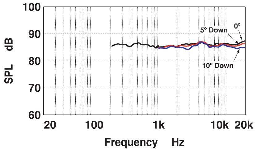
Fig. 4: Vertical off-axis frequency responses below axis.
