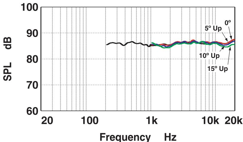
Fig. 3: Vertical off-axis frequency responses above axis.
