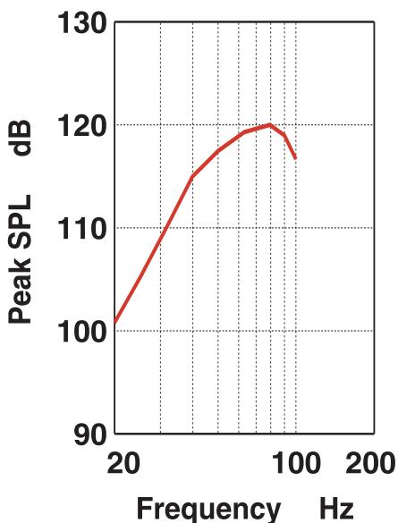
Fig. 8: Woofer maximum peak SPL vs. frequency.
