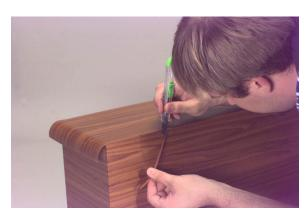
12. Once the cabinet is completely covered, carefully trim the vinyl around the driver and terminal cutouts. The fine-point razor knife will be very handy for following the curves of the cutouts.
