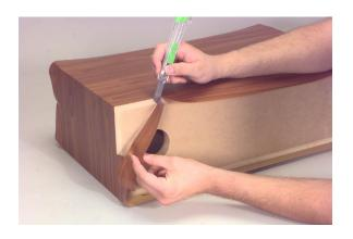
10. Once the sides have been trimmed flush, prepare to install the front and rear pieces of vinyl.
