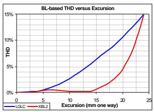
shown above,  $XBL^2$  typically **adds** excursion to a given set of parts, thus leading to even lower distortion for motors based on those parts.
