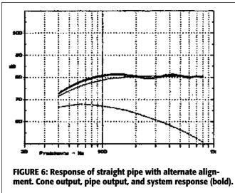
are typical of what you can do with a basic transmission line. Efficiency is 2-5dB less than a comparable closed box, no matter which low-frequency rolloff you prefer. Fortunately, as I will show in Part 3, it is possible to improve the situation by building something other than a simple straight pipe.
