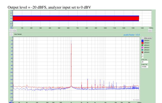
Interestingly the distortion of the voltage output circuit is lower than the distortion of the current mode output circuit at this level.
