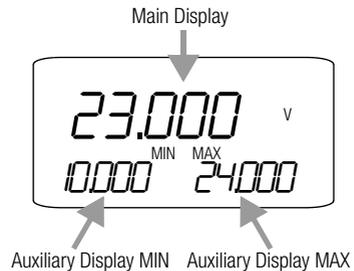
The main display appears immediately after the multimeter is switched on, but the auxiliary displays have to be activated by pressing the DATA/CLEAR key (except for position M $\Omega$ @...V, where the auxiliary displays appear immediately upon selecting the function).
