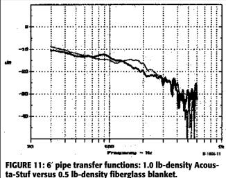
Which material is best? Each one shows deviations from ideal damping characteristics, and even with closematching, these deviations may be audible. However, there are other factors to consider, such as consistency, availability, and ease of handling.
