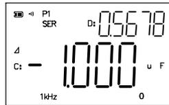
Figure 4-5 Absolute deviation ( $\Delta$ ) display mode
