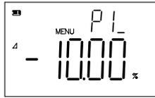
Figure 4-7 Sorting Limit Setup
