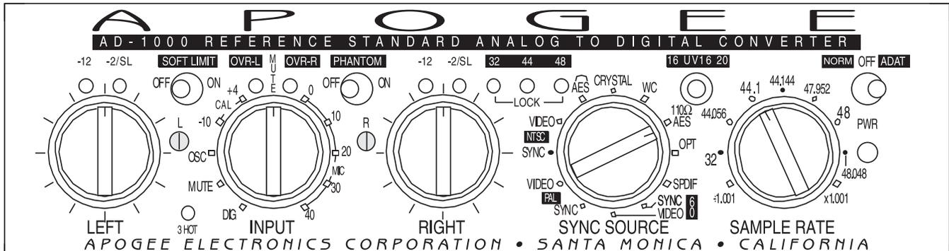
The AD-1000 offers an input section that can receive a wide variety of Analog and Digital inputs ranging from low microphone levels to the hottest line levels. The controls affecting the audio input selection and level are located toward the left of the unit and are detailed above. AES, S/PDIF electrical and optical signals can also be input and reformatted to other digital output types.
