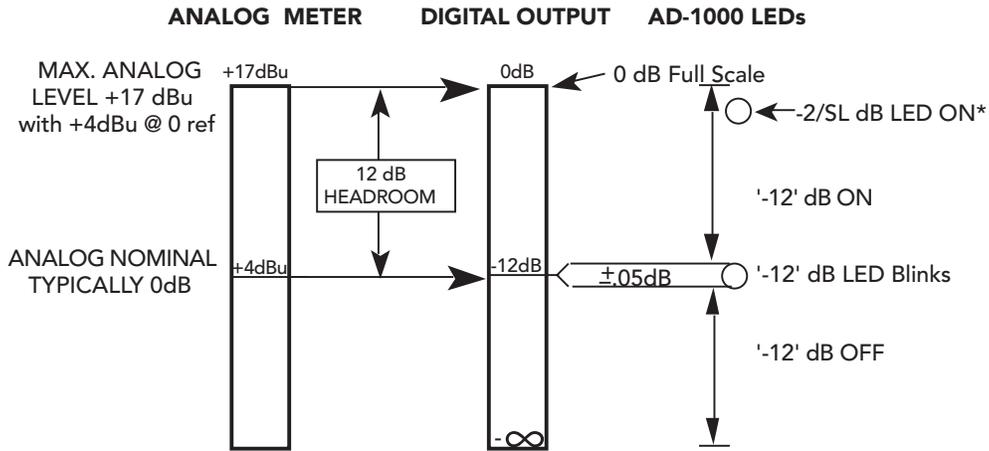
COMPARISON OF ANALOG INPUT TO DIGITAL OUTPUT WITH 12dB HEADROOM AND +4 dBu REFERENCE
