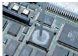
Thermal interface for CPUs
