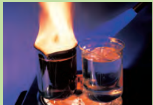
Heat resistance comparison (Left: mineral oil Right: silicone fluid)
