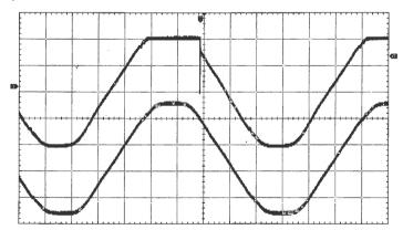
Figure 3 Secondary voltage in Fig.2 supply. Lower: unloaded. Upper: 1N5262GP + 100mA load. 10V/div, 2ms/div.
