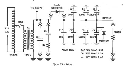
A 600 watt autotransformer ("Variac") connects the test fixture to the AC mains, allowing fine-tuned adjustment of the output voltage. The Variac drives the primary of the power transformer X1 (115V primary, 24V secondary) through a 1 amp, fast-blow fuse. X1's secondary drives the diode (DUT) and, if
