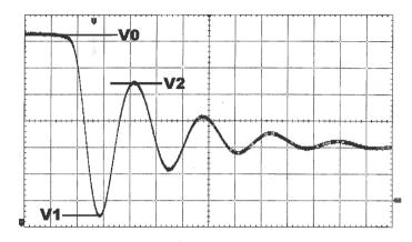
Figure 4 SBR12A45 at 100mA dc load current. Initial step down amplitude "V01" is 6.60V; first ringing amplitude "V12" is 4.88V. (Cursors + legend omitted). 1V/div, 5us/div.
