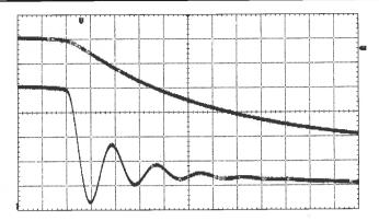
Figure 8 HEXFRED HFA08TB60 at 100mA. Lower (no snubber): V01=4.70V, V12=2.41V. Upper (with CRC snubber): no ringing. 1V/div, 5us/div.
