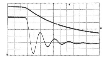
Figure 10 Schottky diode SB540 at 100mA. Lower (no snubber): V01=5.28V, V12=3.14V. Upper (with CRC snubber): no ringing. 1V/div, Sus/div. Soft Recovery Diodes Lower Transformer Ringing by 10-20X
