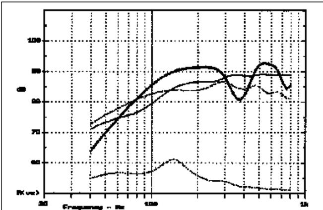
**FIGURE 4A:** Response of loudspeaker on straight pipe with light damping. Impedance, cone output, pipe output, and system response (bold).
