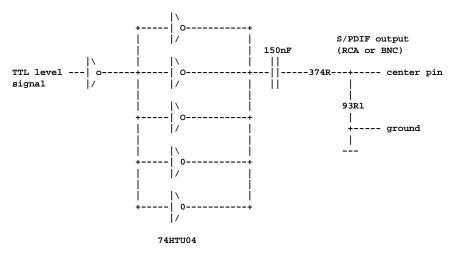
This circuit does not provide any isolation on the output. The TTL level signal form 74HCT04 buffer is attenuated to the levels specified in S/PDIF optical interface by using the voltage divider made of 374 ohm and 93.1 ohm resistors. This circuit is based on S/PDIF converter circuit diagram from Elektor Electronics magazine issue 4/1997 page 66.
