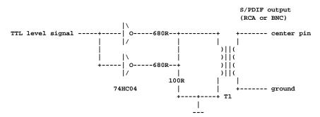
Idea for this circuit is taken from "A digital Output for the CD720" web page (was at <u>http://www.spiceisle.com</u>/homepages/brian/audiodiy/mods/digi-out.htm). The transformer T1 is high quality 1:1 pulse transformer (can be salvaged from old broken network interface card or similar source).
