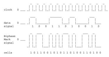
The frequency of the clock if twice the bitrate. Every bit of the original data is represented as two logical states, which, together, form a cell. The length of a cel ('time-slot') is equal to the length of a databit. The logical level at the start of a bit is always inverted to the level at the end of the previous bit. The level at the end of a bit is equal (a 0 transmitted) or inverted (a 1 transmitted) to the start of that bit.
