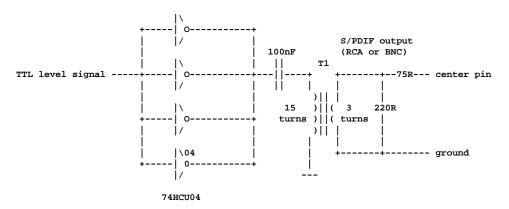
This circuit is part of circuit "Splitter for S/PDIF coax/optical output" by T. Giesberts from Elektor Electronics magazine July/August 1995 pages 78-79. The transformer T1 is made to G2.3-FT12 ferrite ring core. Primary coil is 15 turns of 0.5 mm diameter enamelled copper wire and secondary is 3 turns of 0.5 mm diameter enamelled copper wire. The chip 74HCU04 is manufactured by Philips
