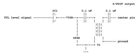
T1 is a HF-transformer which has 2:1 turns ratio. Transformer type used in example circuit is SC944-05. IC1 in this circuit consists of 8 parallel connected buffer ports from 74ACQ244 IC.
