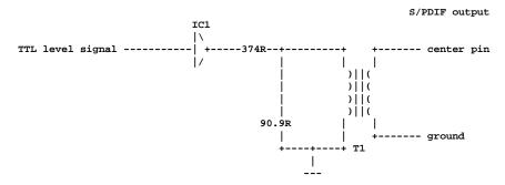
The transformer used in this circuit is 1:1 pulse transformer (the original application note suggested pulse transformer from Pulse Engineering or Schott Corporation). IC1 is a buffer IC which must be capable to supply enough current to drive the 75 ohm S/PDIF interface to full votlage swing specified (capable of loading 415 ohm load or capable of supplying 12 mA current).
