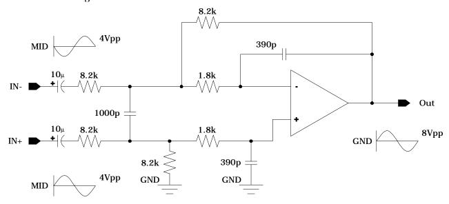
Differential to Single-ended Converter and 2-pole 48kHz lowpass filter
