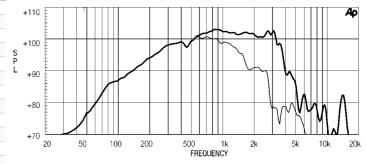
FREQUENCY RESPONSE CURVE OF 12MB1000 MADE ON 50 LIT. CLOSED BOX ENCLOSURE IN FREE FIELD (4PI) ENVIRONMENT. ENCLOSURE CLOSES THE REAR OF THE DRIVER. THE THIN LINE REPRESENTS 45 DEG. OFF AXIS FREQUENCY RESPONSE FREE AIR IMPEDANCE MAGNITUDE CURVE
