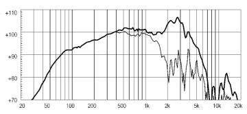
FREQUENCY RESPONSE CURVE OF 12MB700 MADE ON 50 LIT. ENCLOSURE TUNED 60HZ IN FREE FIELD (4PI) ENVIRONMENT. ENCLOSURE CLOSES THE REAR OF THE DRIVER. THE THIN LINE REPRESENTS 45 DEG. OFF AXIS FREQUENCY RESPONSE
