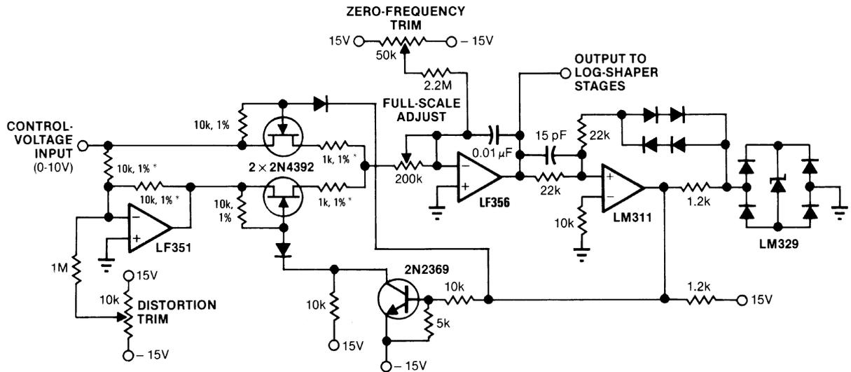
Adjust distortion for minimum at 1 Hz to 10 Hz
