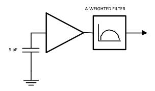
Figure 23. Noise Measurement Setup
