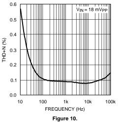
Total Harmonic Distortion vs. Frequency (LMV1012-25)
