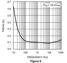
Total Harmonic Distortion vs. Frequency (LMV1012-20)
