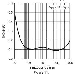
Total Harmonic Distortion vs. Frequency (LMV1012-15)
