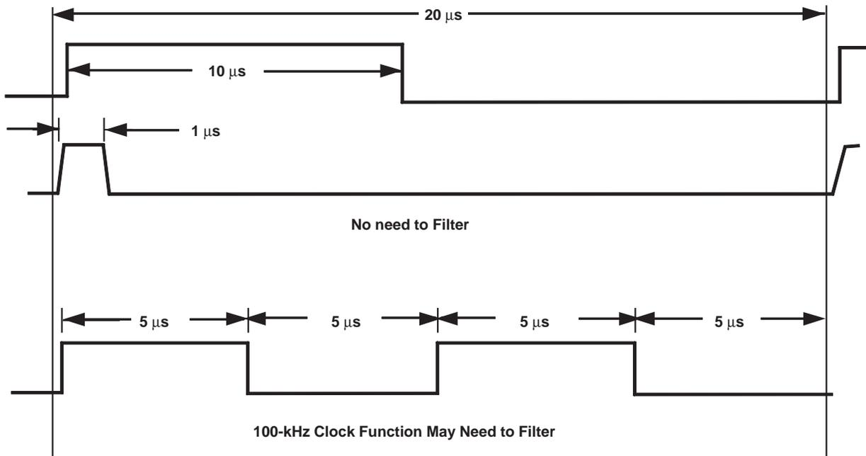
**Figure 1. Signals Below 50 kHz Are Not EMI Concerns**
