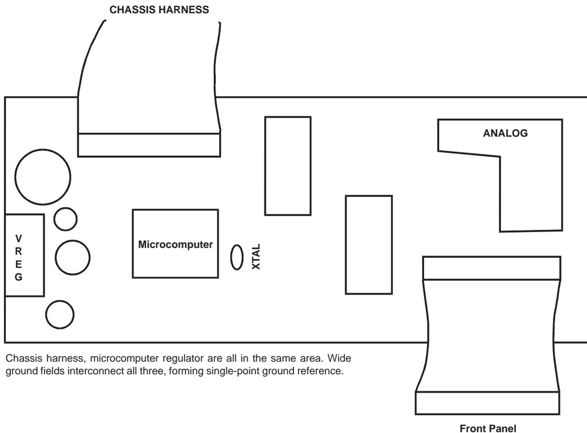
Chassis harness, microcomputer regulator are all in the same area. Wide ground fields interconnect all three, forming single-point ground reference.
