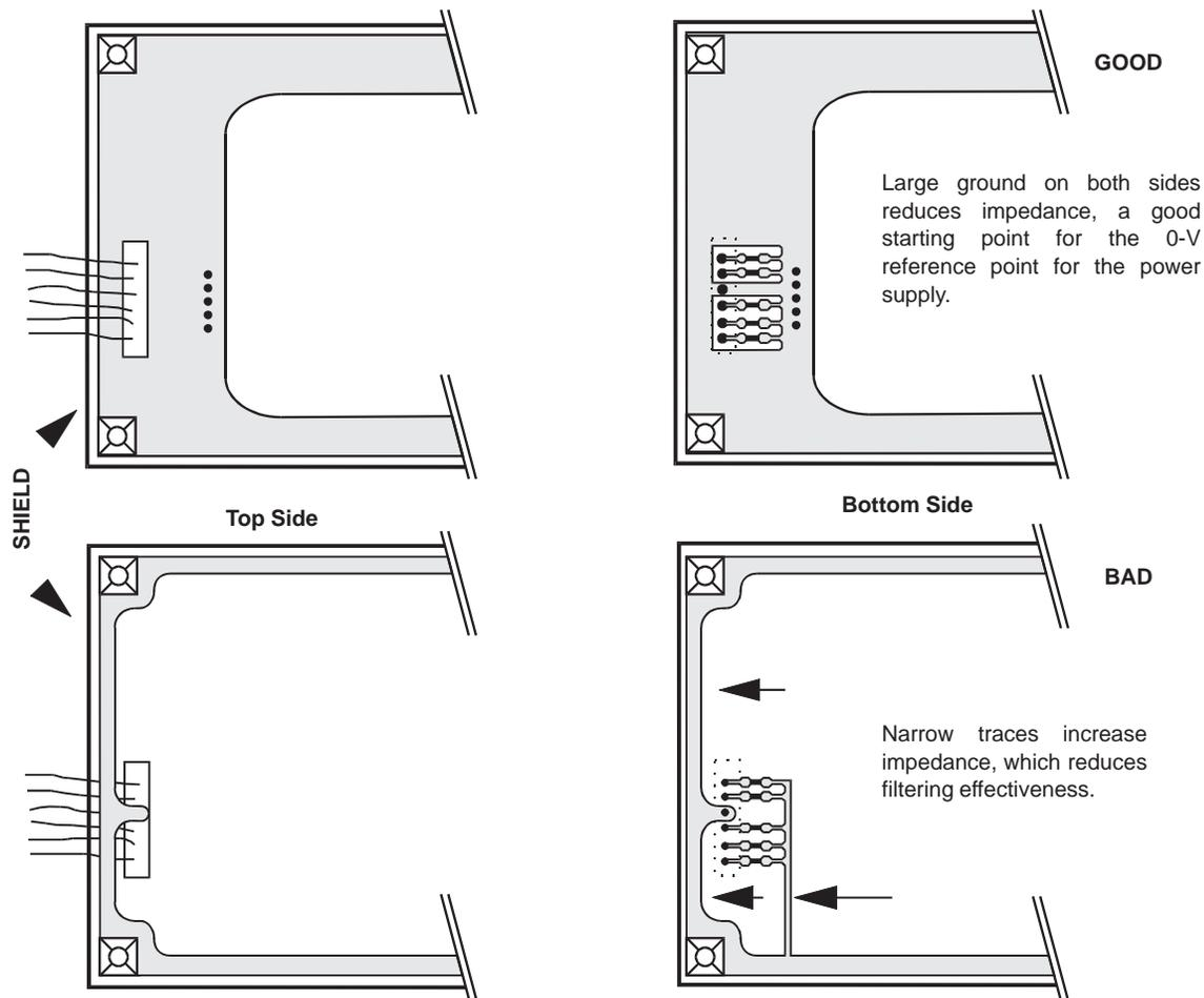
Figure 13. Mounting Filter Capacitors for External I/Os
