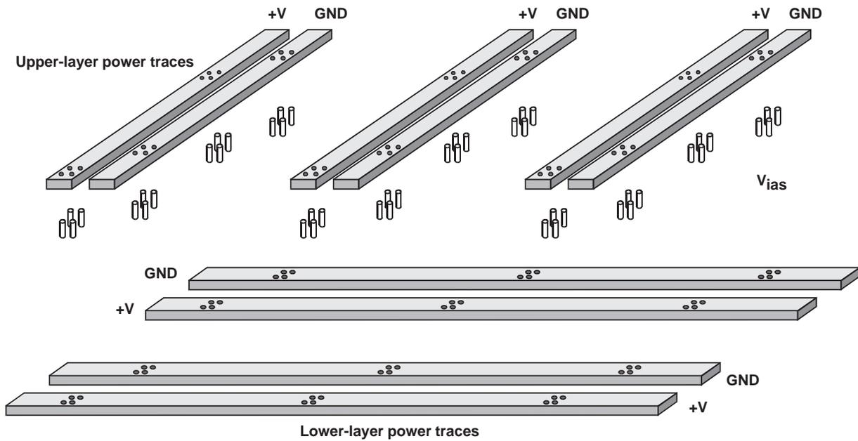
**Figure 7. Gridding Power Traces on Two-Layer Boards**
