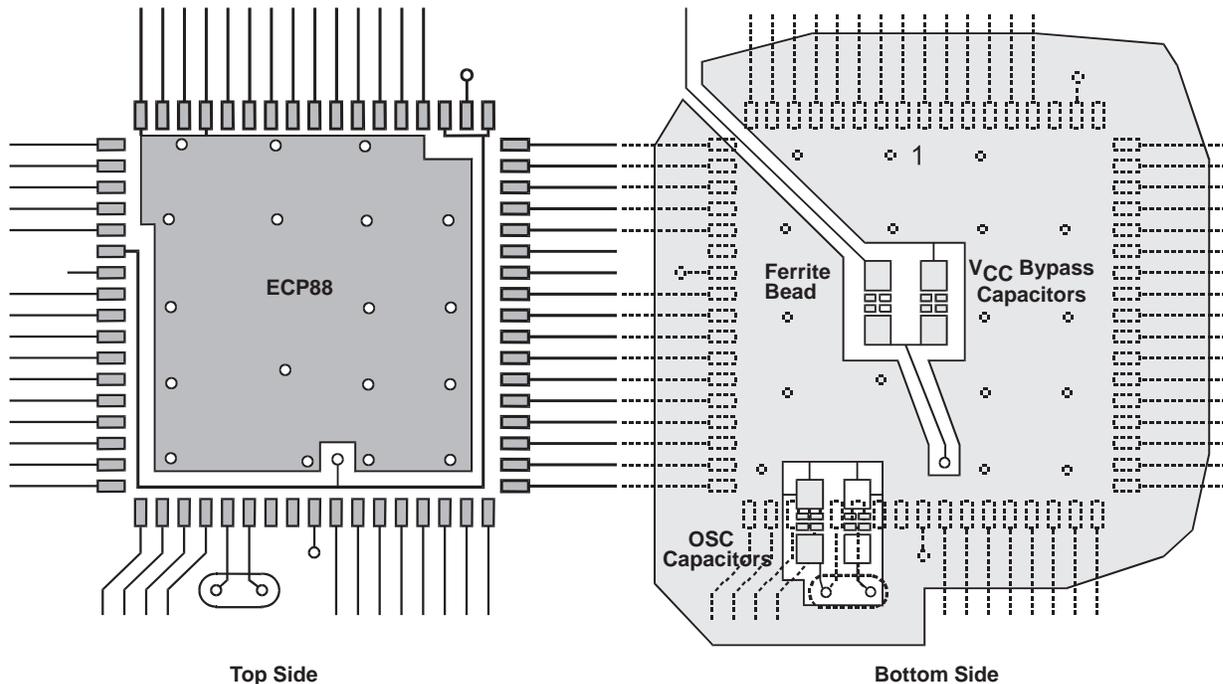
Figure 4. Microcomputer Ground
