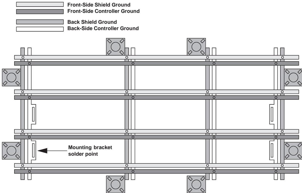
**Figure 12. Front-Panel Gridding to Form Two Ground Planes**
