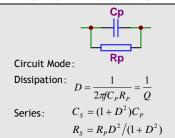
Capacitance Cs: from series to parallel
