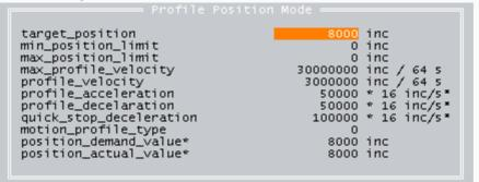
Now we set the *target\_position* to 8000 if *profile\_velocity* equals 0, nothing happens and we set the *profile\_velocity* to 3 000 000 (350 U/min).
