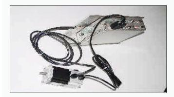
The motor encoder uses signals according to RS422. The encoder is supplied with 5 V by the controller at input X8.
