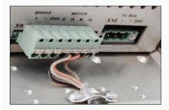
The wiring system of X9 you find in the table below. The values in brackets are in case you are using female connectors. The ground cable and shield should be well mounted on the controller (see picture above). Over 60 VDC the GND-lead is needed.
