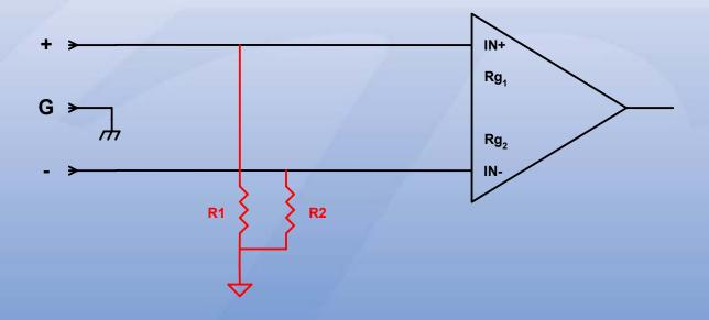
Must provide a DC current path to supply the amplifier input bias current
