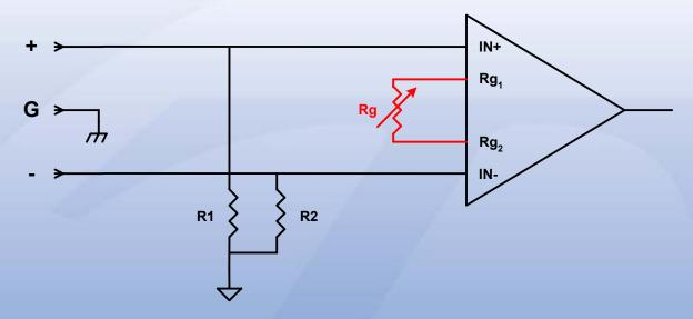
The amplifier is often designed to vary gain using a single variable resistor (R<sub>g</sub>)
