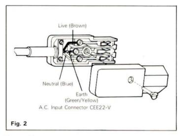
A.C. input is via a standard CEE22-V plug and socket. The amplifier chassis must be connected to ground via the A.C. supply cord. A simple retaining clip ensures that the A.C. connectors cannot be removed by accident.
