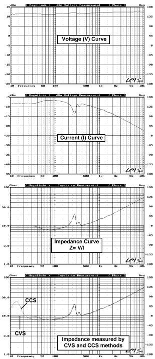
loudspeaker under the same drive conditions and levels as will occur during normal operation. It is not at all uncommon to see a significant difference between CCS and CVS measurements. In this example the impedance data taken using the simple CCS method would be grossly inaccurate at low frequencies, relative to the normal operation of the speaker.
