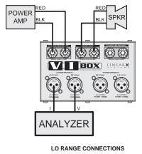
**Warning!** Exceeding the current limit of 2.5A in the low range will cause the current shunt to burn out! Please make sure to use the high power (25A) range for higher power measurements.
