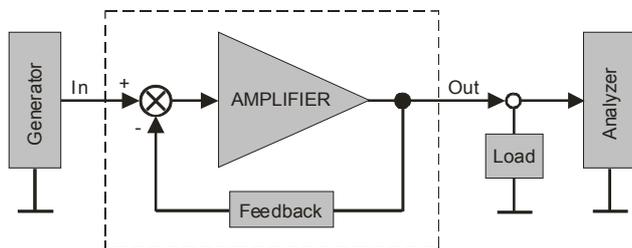
Fig. 7. Circuit for measurement of amplifier parameters
