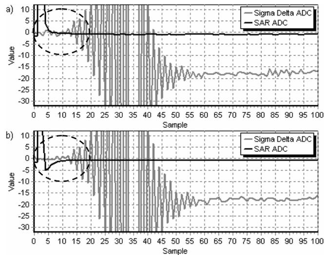
Fig. 8. Load influence on power amplifier work, a) without load, b) with resistant load
