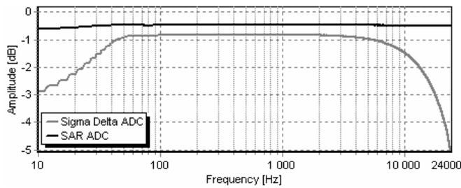
Fig. 6. Calculated frequency responses of two ADC types
