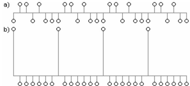
Fig. 1. Example of MLS (a) and its autocorrelation (b) for  $M = 7$
