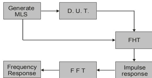
Fig. 2. Block diagram of MLS algorithm
