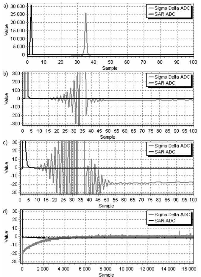
Fig. 5. Calculated impulse response of two types of ADCs
