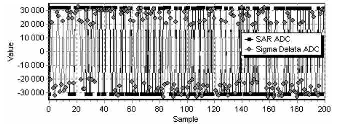
Fig. 4. Acquisition MLS by SAR and Sigma-Delta ADC
