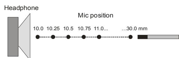
Fig. 10. Method of headphones SPL measuring
