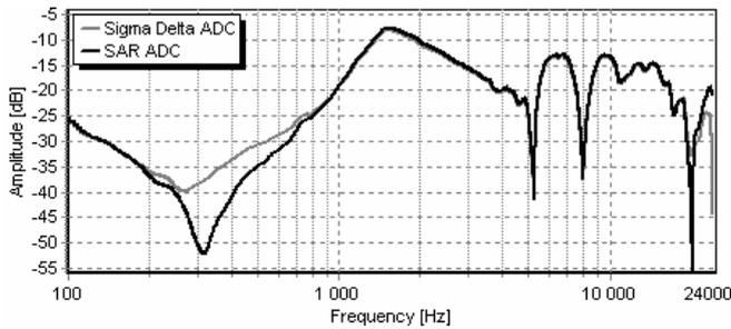
Fig. 11. Different SPLs measured by two types of ADCs
