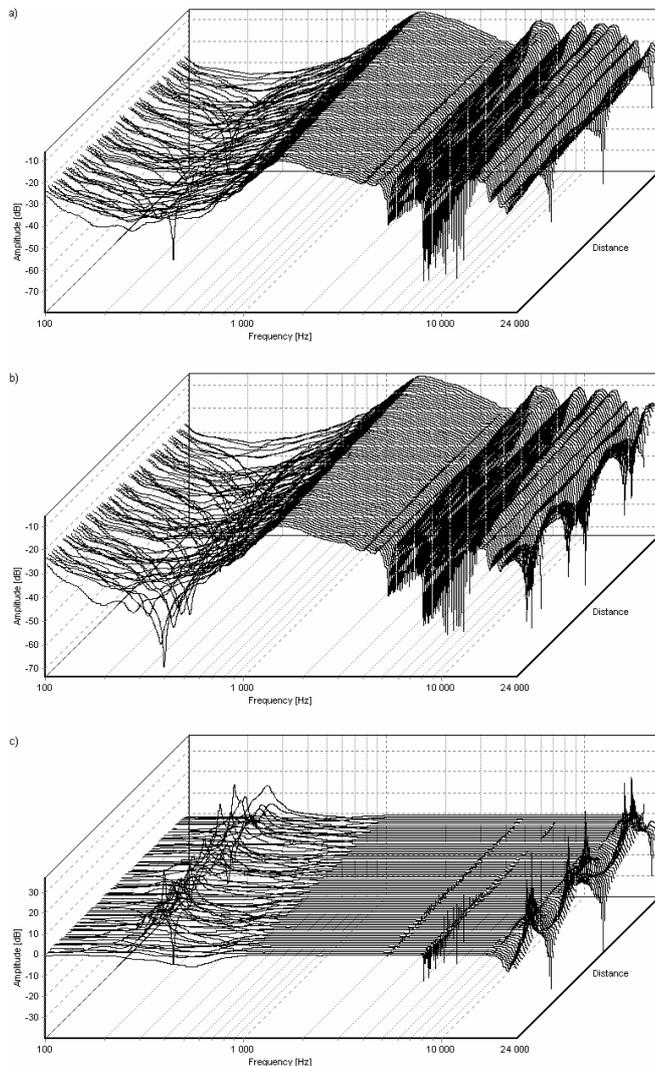
Fig. 12. Headphones frequency response in different distance, a) for sigma-delta ADC, b) for SAR ADC, c) the difference
