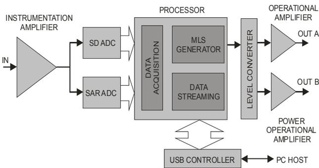
Fig. 3. Block diagram of dual ADC board
