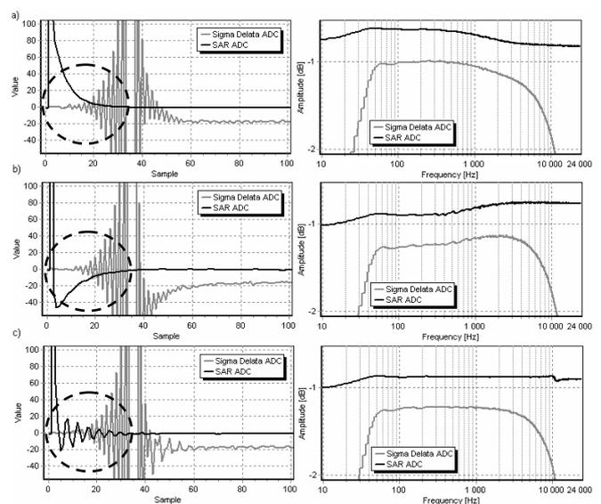
Fig. 9. Load influence on power amplifier work, a) resistance-capacitance load, b) resistance-inductance load, c) resistance-inductance-capacitance load
