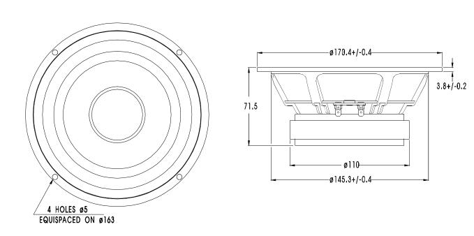
P17REX is a 6,5" High Fidelity woofer with an injection moulded metal chassis. A polypropylene based cone, a soft PVC dust cap and a high loss rubber surround are carefully matched to each other, resulting in an outstandingly smooth frequency response. The unit has a high power handling capacity due to its relatively large voice coil diameter. The magnet system has a T-shaped cross section of the pole piece for low modulation distortion. A large magnet system provides high efficiency and low Q.
