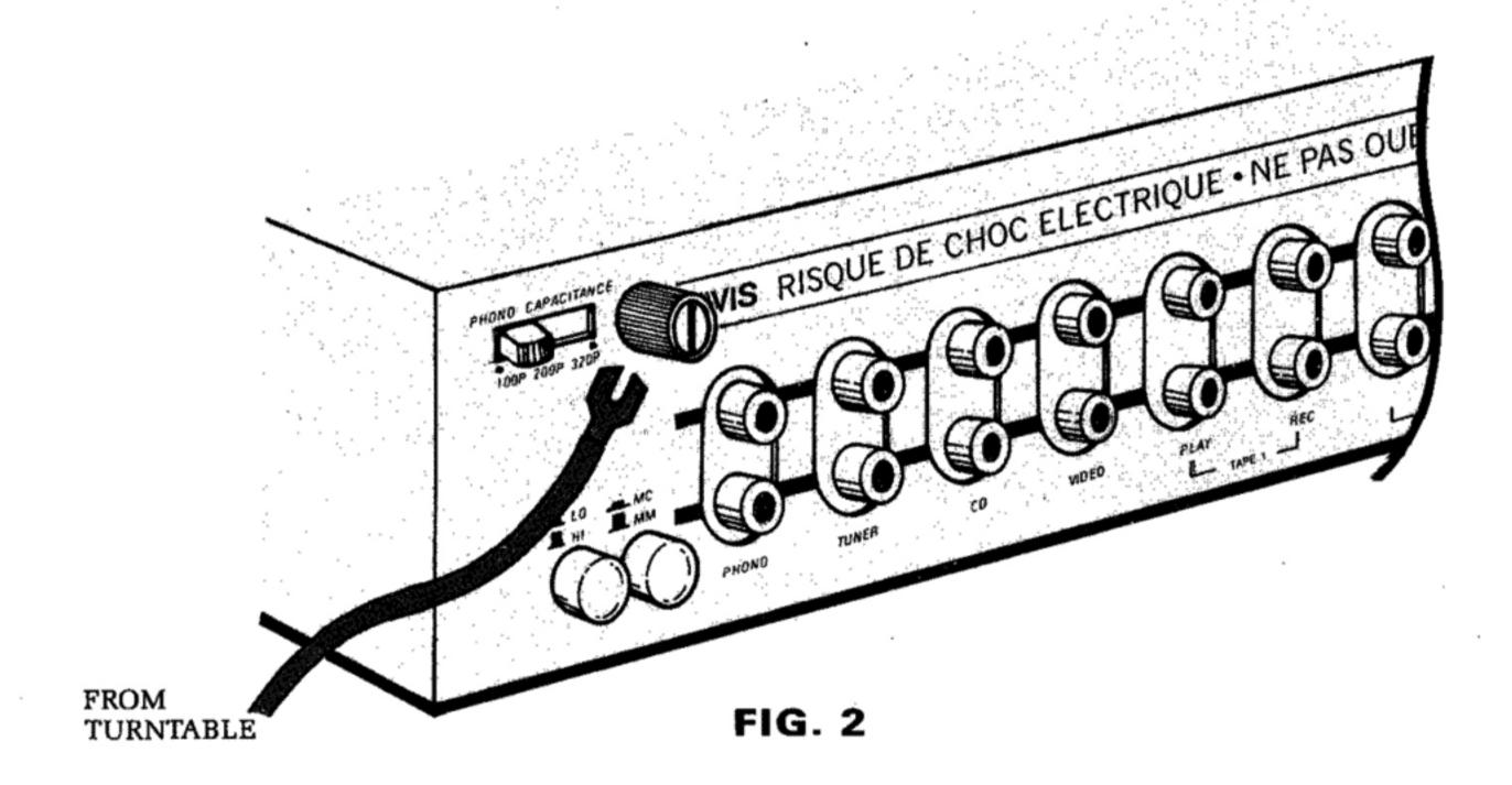
ground cable to the P1100 GROUND terminal (1) in the following manner:
