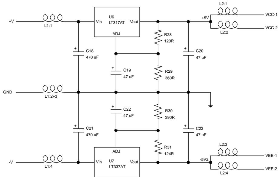
+V and -V can normally be stolen from the player's power supply. Most players have unregulated power rails of about +9V or +11V and -9V or -11V. Make sure that the power is taken before any kind of current limiters.
