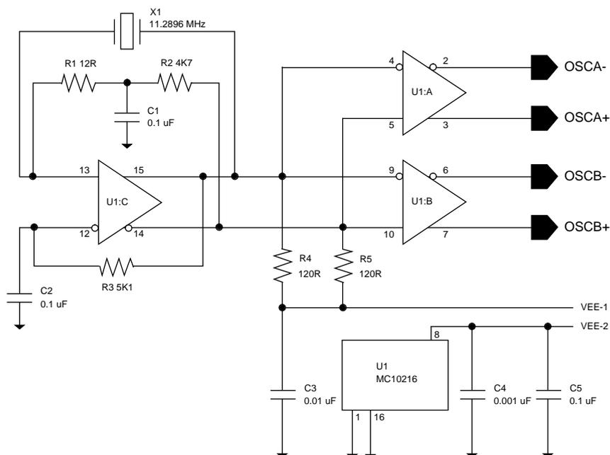
R1 should match the equivalent series resistance of the crystal. So for e.g. a 16 MHz crystal R1 should be changed from 12R to 10R.
