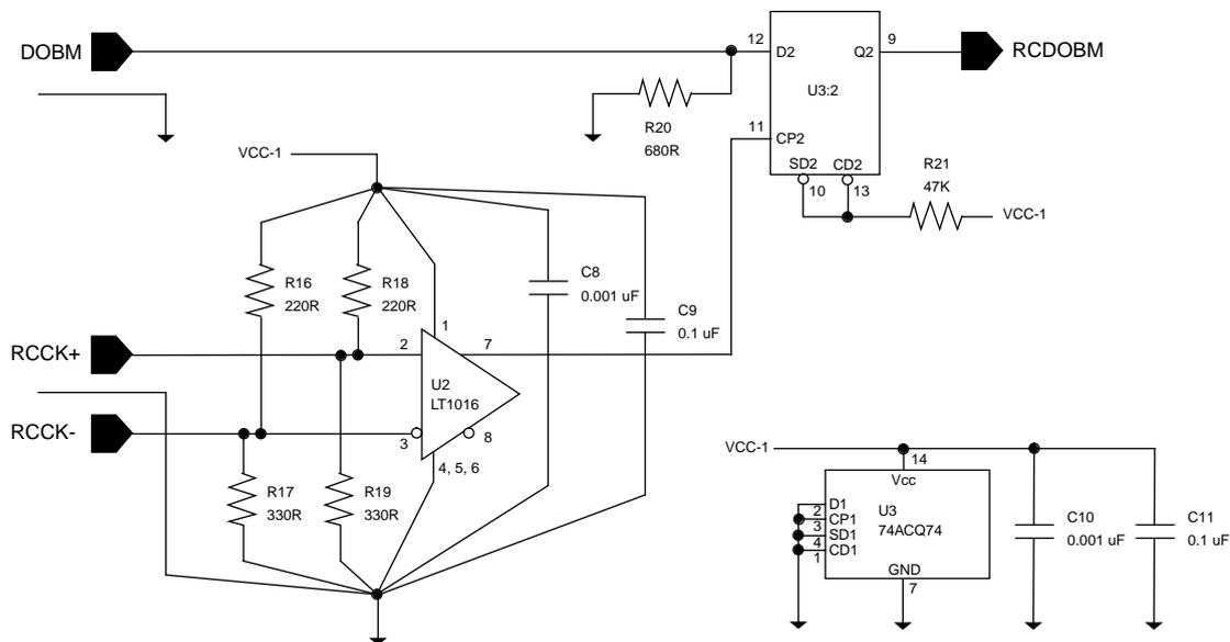
To insure good operation of the reclocker, make sure that the data on D2 is stable 10 ns on both sides of the rising clock edge on CP2. If it isn't stable, invert the SYSCK as described later.
