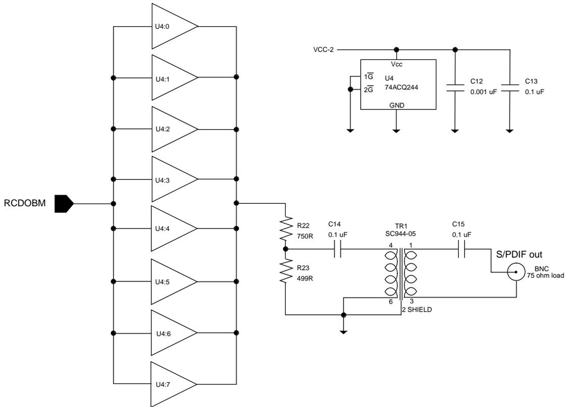
Note: Impedance matching is based on that the HF-transformer is of type 2:1. So if for some reason a 1:1 transformer is used as a replacement, the resistor values have to be recalculated.
