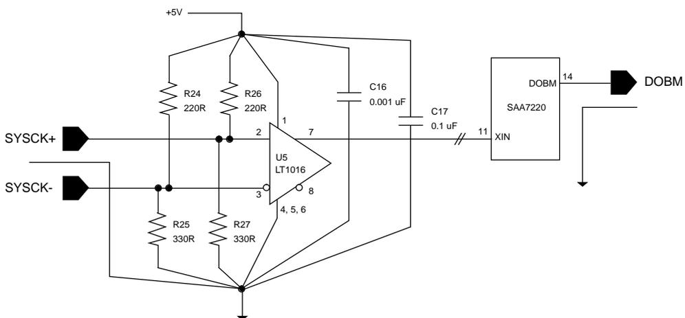
The above interface circuitry should be mounted close to the XIN on the SAA7220. The crystal oscillator in the player must also be disabled. This is often a 11.2896 MHz crystal, a resistor and two capacitors around pin 10 and 11 on the SAA7220. It is also a good idea to disable everything that might be connected to pin 14 on the SAA7220.
