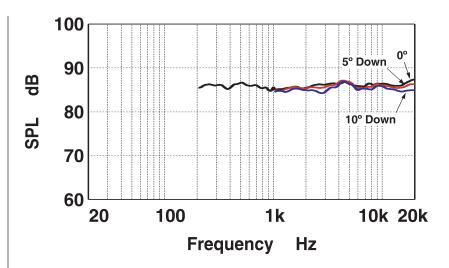
Fig. 4: Vertical off-axis frequency responses below axis.
