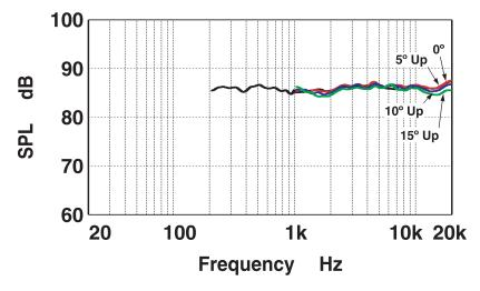
Fig. 3: Vertical off-axis frequency responses above axis.
