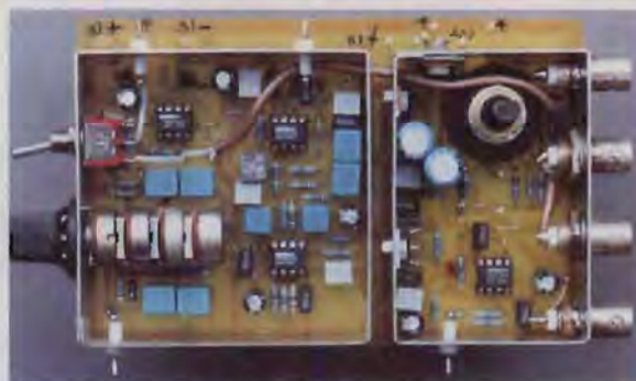
Figure 2: The higher power 100Hz test system. Four BNC connectors are arranged to accept Hewlett Packard test fixtures. The DC bias network inserts between the buffer amplifier and test fixture.
